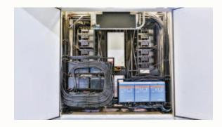
Ingenious engineering, world wide unique concepts and a specially developed server rack allow the integration of highly sensitive IT-systems into a vehicle that is continuously exposed to vibrations and shocks. Our unique suspension system ensures that there is no damage to the special electronic components whilst on the move!
